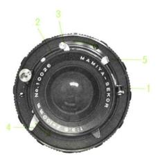
CABLE RELEASE: Screw the cable release into the cable release socket (1). SHUTTER SPEED: Rotate the shutter speed ring (2) until the desired shutter speed scale is aligned with the index mark.
